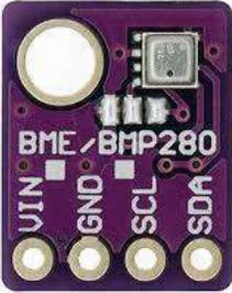
A purple PCB module for the BME/BMP280 sensor. It features a white circular sensor lens, a microcontroller chip, and four pins labeled VIN, GND, SCL, and SDA.                 |
